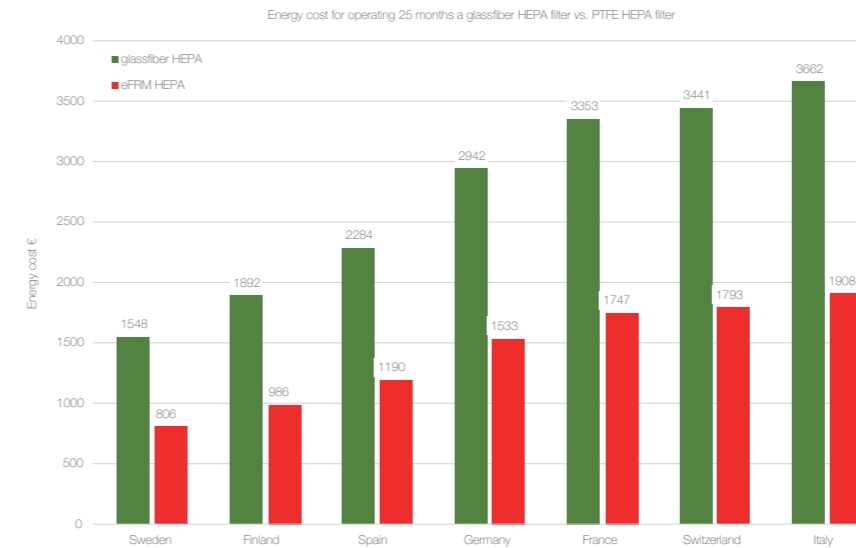
Figure 5: Energy cost for operating glassfiber HEPA filter vs. eFRM membrane HEPA filter in different countries.
